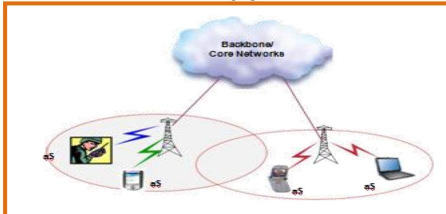
Figure 3. Infrastructure-based network architecture[22]
